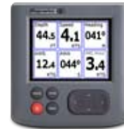
Customize the display with analog, digital, bar graphs and historical data displays
