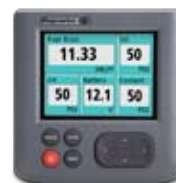
Engine instrumentation using NMEA2000
